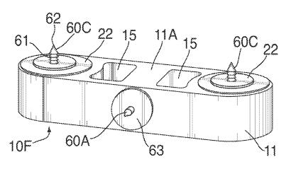
the dimensions of the neuroforamen through which it typically passes to be deployed within the intervertebral space. The implant is provided with a locking system having a plurality of linked locking elements that work in unison to lock the implant in an extended configuration. Bone engaging anchors also may be provided to ensure secure positioning.
